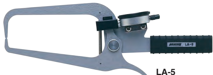
LA-5 Graduation: 0.05mm Range: 0~50mm Throat depth: 150mm
