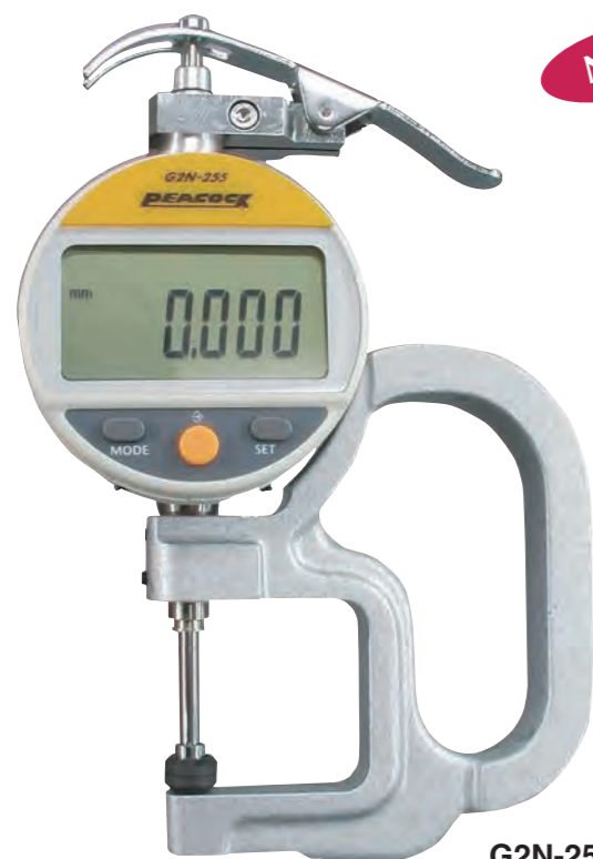
G2N-255 Range: 20mm Resolution: 0.001mm
