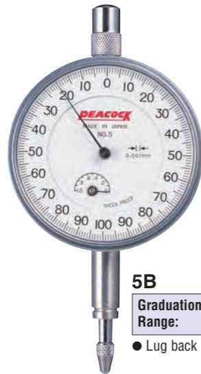
5B-HG Graduation: 0.001mm Range: 1mm ● Indication error \pm 3\mu\text{m} ● Retrace error 2\mu\text{m} ● Includes accuracy certification ● Lug back
