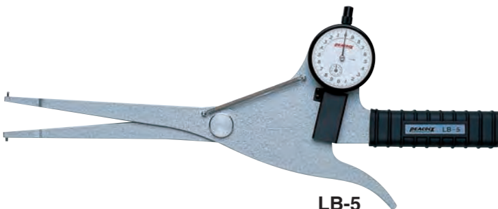
LB-5 Graduation: 0.01mm Range: 20~40mm Throat depth: 150mm
