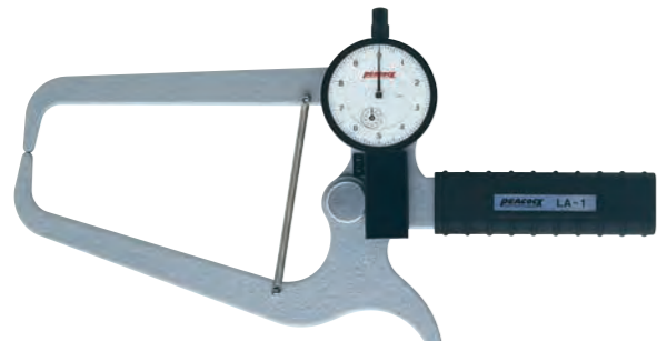
LA-1 Graduation: 0.1mm Range: 0~80mm Throat depth: 120mm
