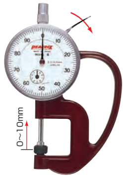
G Graduation: 0.01mm Range: 0~10mm
