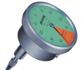
196Z Graduation: 0.01mm Range: 0.8mm ● Stem \phi 8mm ● Pointer giving less than one revolution ● Contact point (X-112)
