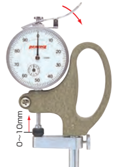
G-3 Graduation: 0.01mm Range: 30mm
