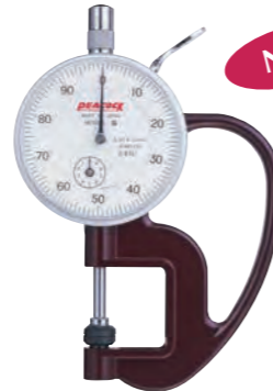
G-2.4N Graduation: 0.01mm Range: 0~10mm
