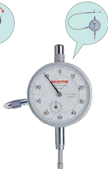
107-BL Graduation: 0.01mm Range: 10mm ● Spindle pull-up back lever ● Lug back
