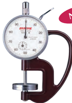
G-30 Graduation: 0.01mm Range: 0~10mm
